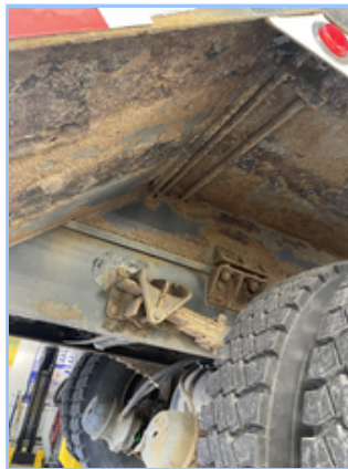
Corrosion on WW Screenings truck
